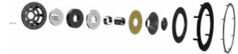
A precision-made magnet system with an aluminium compensation ring to minimise the effect of variations in inductance as the voice coil travels. This contributes to an absence of distortion and intermodulation generated by the 'motor system'.
