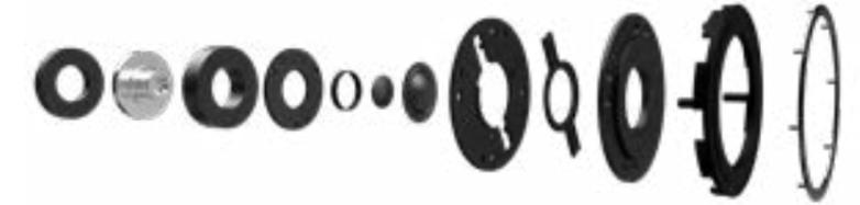
The 25mm dome is made from a woven polyester film with a high-loss coating to deliver open and smoothly extended high frequencies. The magnet system and the front plate have been optimised for wide dispersion and uncompressed behaviour. The front plate is flat and exposes the dome as much as possible; only a very short duct on the front plate balances the acoustic load and improves the SPL (sound pressure level) measurement.
