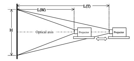
Image of height H is projected in the range from the shortest distance L (W) to the longest distance L (T).
