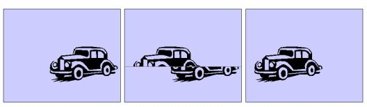
In this example, a composite image appeared when an object moved from right to left, which is a combination of the frames before and after the movement.
