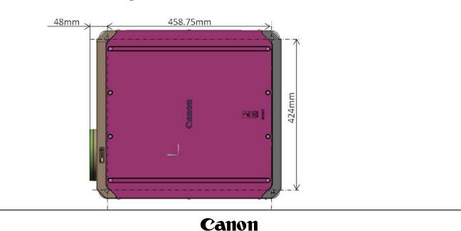
Screw holes for ceiling mount: 4 (M6)
